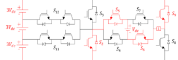
Fig. 3.1(xxii) Equivalent Circuit of Mode 22
